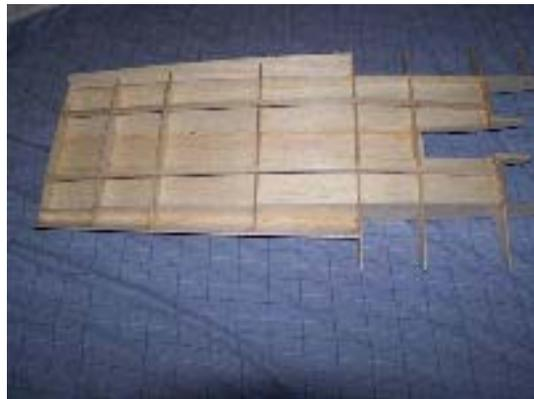
gluing the deck on you can remove twist by ensuring everything is flat on the building board before gluing. i.e. same contact points!
